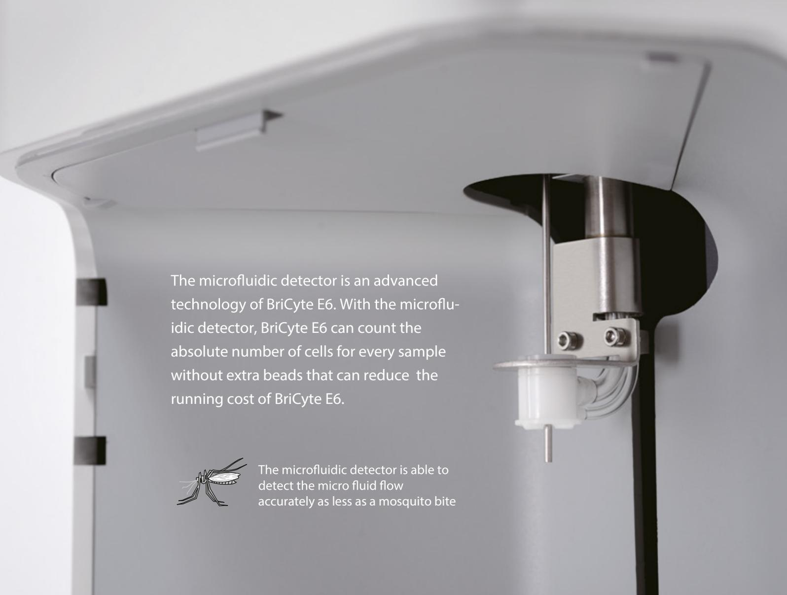
The microfluidic detector is an advanced technology of BriCyte E6. With the microfluidic detector, BriCyte E6 can count the absolute number of cells for every sample without extra beads that can reduce the running cost of BriCyte E6.
