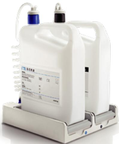
The sheath fluid and waste could be placed on the weight sensors which are able to measure the residual volume of reagents. With such design, the BriCyte E6 can sound an alarm before the reagents run out to minimize the dead volume.
