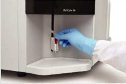
BriCyte E6 has open mode which suits the labs which have less number of samples, the micro sample tubes are supported as well. The carousel mode is yet another option which can handle 40 sample tubes at one time.
