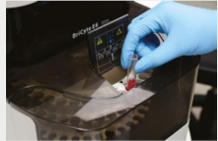
In the carousel mode, single sample tube can also be loaded as STAT after opening the cap of carousel.
