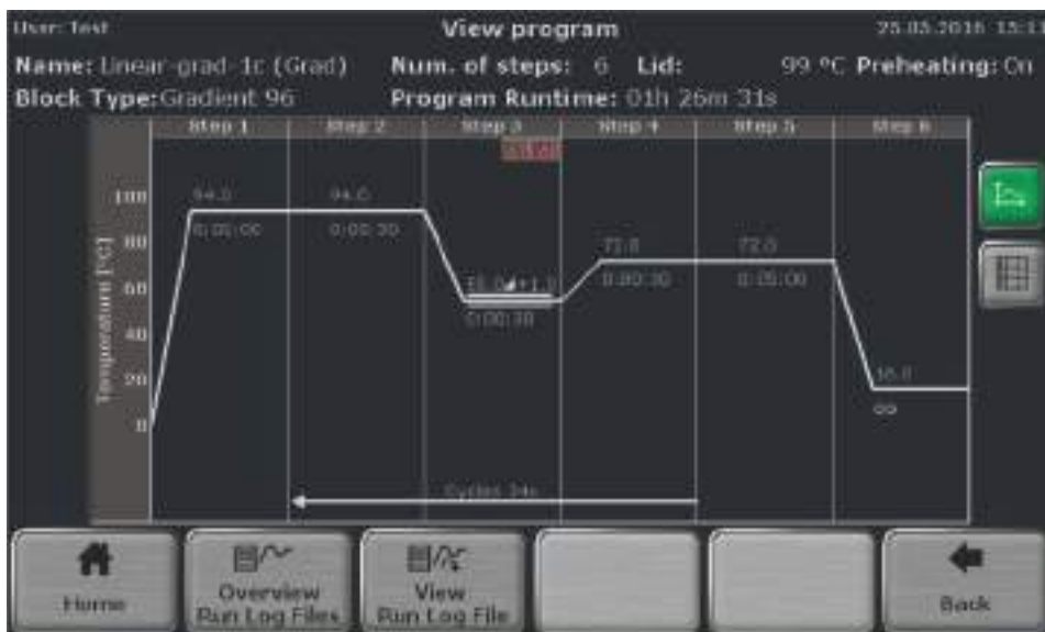
Figure 56. QIAamplifier 96 program view screen.
