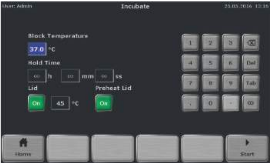
Figure 14. QIAamplifier 96 incubation mode screen.
