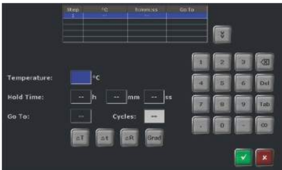
Figure 21. QIAmplifier 96 program step editing screen.
