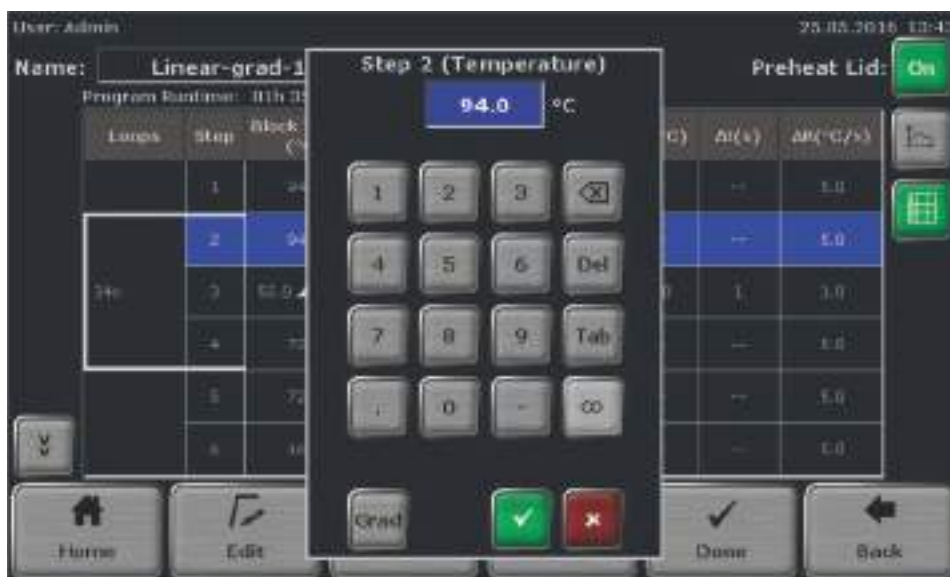
Figure 27. QIAmplifier 96 individual program parameter editing.
